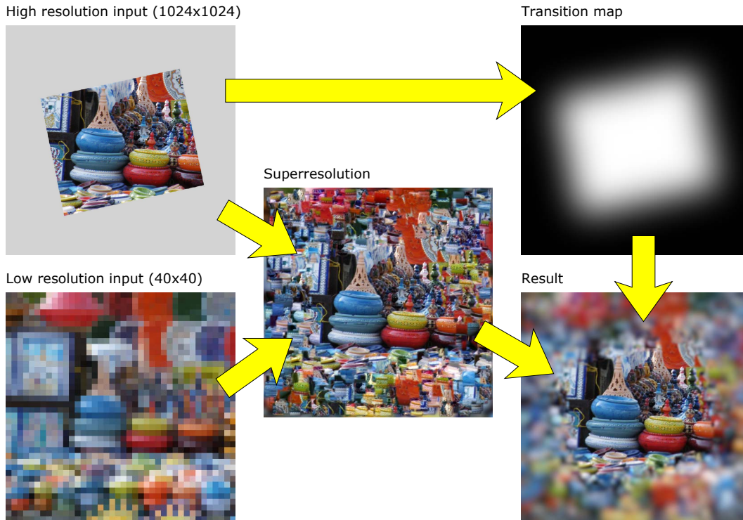
Figure 2: Transition generation workflow. Aligned and photometrically corrected low resolution and high resolution images are the input images on the left. The center shows an intermediate result where high resolution patches have been copied to areas with similar low frequency content. The transition map is derived from the blurred alpha mask of the high resolution input image and controls the amount of blur. The final result is shown on the bottom right.
